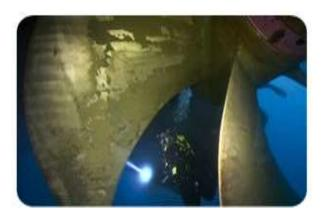
For underwater ship hull inspection, hull cleaning, and propeller polishing reach us at survey@sigma-asia.com or WhatsApp +65 96602617 (24/7) However, in terms of energy loss per unit area, propeller roughness significantly affects ships fuel consumption as well. Therefore, higher standards of propeller maintenance can be more cost effective than hull maintenance for many types of ships.
